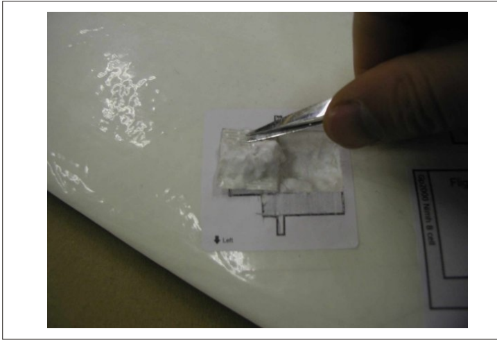
Step 3: Prise out the foam bit by bit, checking with the servo for a nice tight fit. The servo should lie flush with the top surface of the wing.
